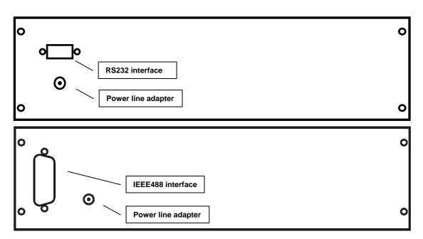
The rear panel contains the power supply connector, interface RS-232 or GPIB connectors and the instrument's label.
