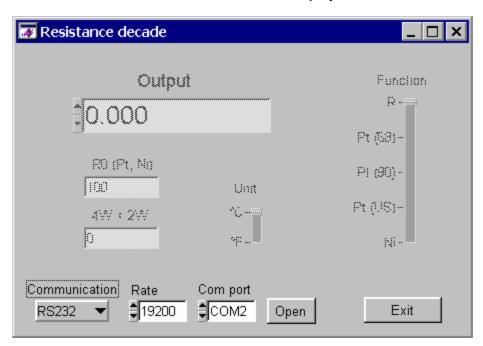
First the "Communication" RS232 or IEEE488 will be selected. For the RS232 the COM and the Baud Rate have to be defined. By using the IEEE488 only the address will be selected. When the key "Open" is activated, the instrument is connected to the data bus and communicates with the PC. The resistance value can be entered with the keyboard into the window OUTPUT. The program can be terminated with the key "EXIT".
