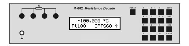
The keyboard, the display and the output terminals are located at the front panel.
